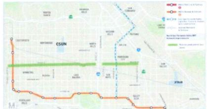
Bus lanes will be installed on Roscoe Bl from Topanga Canyon Bl to Coldwater Canyon Av. The bus lanes will drop between Haskell Av and Sepulveda Bl to accommodate 1-405 freeway ramp operations. The bus lanes will operate in the existing AM/PM peak hour lanes.
